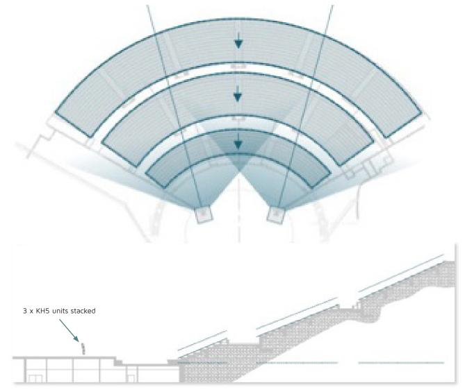
Plan view and sectional view of an amphitheater where two clusters of 3 KH5 are installed
