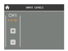
The Levels page allows users to manage the amplitude of the input signal (whether analog or digital).
