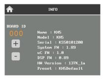
The Info page contains information about the current software and firmware, the current preset loaded and the *Board ID* of the device.
