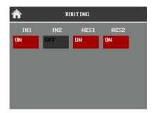
The Matrix page allows users to switch on/off the four inputs channels independently. *IN1* and *IN2* are the two analog inputs, *AES1* and *AES2* are the two channels of the AES/EBU digital input.
