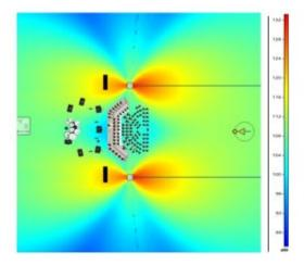
Comparison of the energy distribution of a traditional PA system and a SAT system consisting of 6 KH8 units per side. The simulation shows the SPL values in a third octave band centered at 200 Hz.
